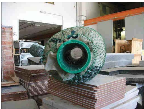
FIGURE 6: drenotube® sample 1, after 6 tests under 0, 3, 6, 9, 12 and 15 kN axial load.
