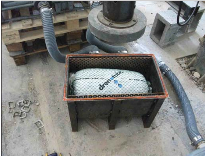
FIGURE 4: drenotube® placed on its isolated box before being tested.
